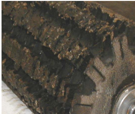
Note that the Magnom's flow channels remain fully clear even when it is fully laden with over 4kg of contaminant
